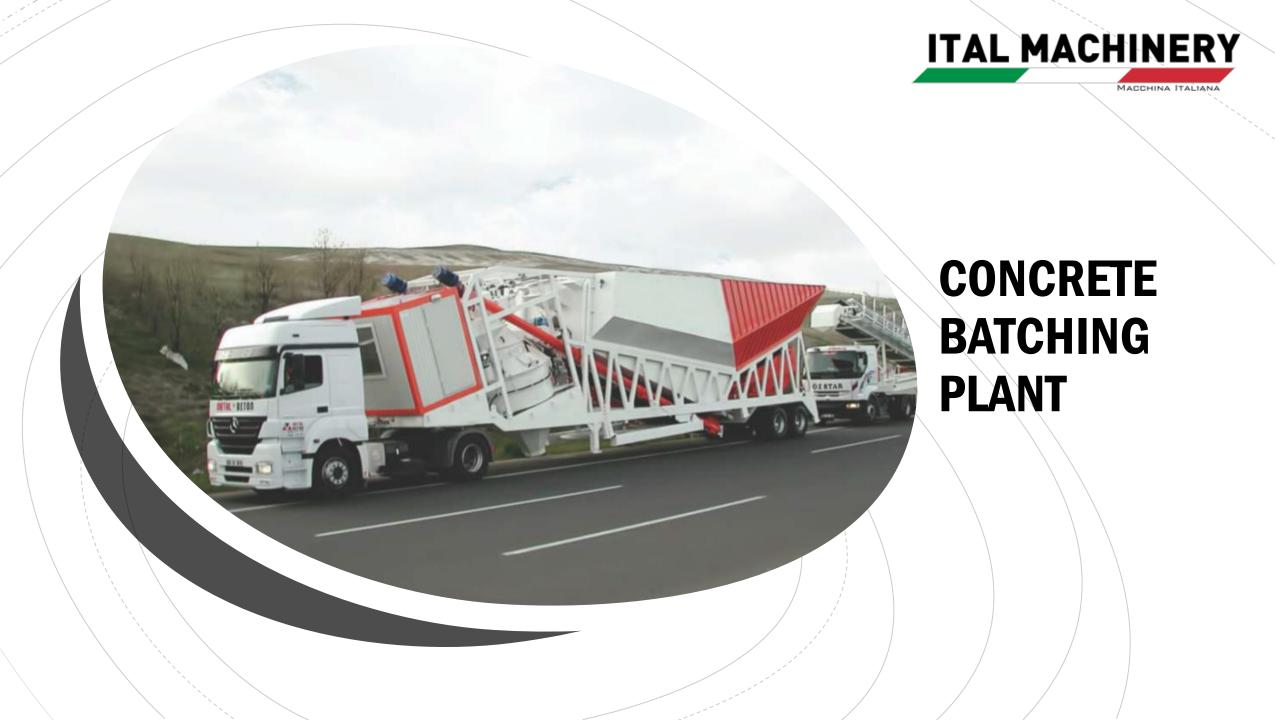
High quality concrete can be produced for all kind of projects where concrete is used by ready mix concrete plants. There are stationary, mobile, compact and on-site type concrete plants available, which can be chosen according to project type, place of use and capacity requirement.
